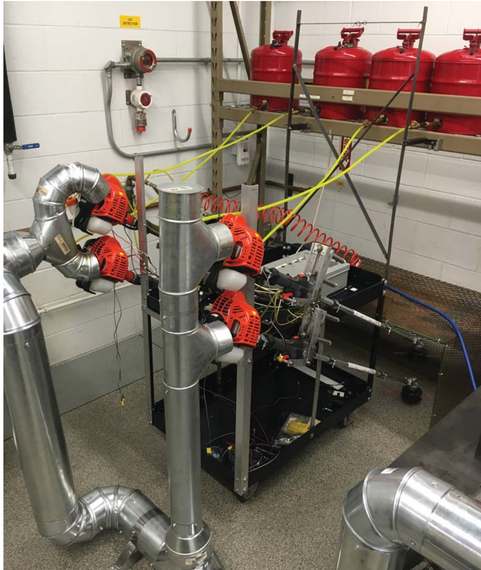
String trimmers arranged on test stand.
