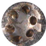
Injector after one P.i. treatment.
