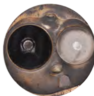
Cylinder head after one P.i. treatment.
