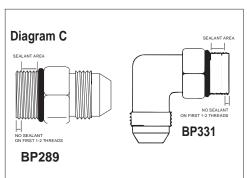
4. Lubricate the O-ring of the BP289 and install in the adapter assembly. If installing into the thread adapter (as in Option 2), tighten to 85ft-lbs. If installing into the side of the filter adapter (as in Option 1), tighten to 56 ft-lbs.
