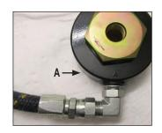
**Note:** Ensure hose has significant additional length to accommodate movement of engine.
