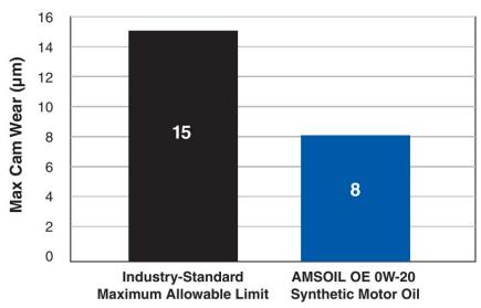
$^*$ Based on independent testing of OE 0W-20 in the Peugeot TU3M Wear Test as required by the dexos1 Gen 2 specification.
