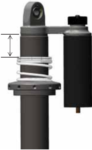
Front Shock Preload Measurement
