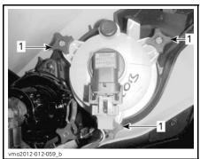
LOW BEAM ADJUSTMENT 1. Adjustment knobs
