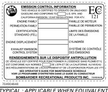
TYPICAL : APPLICABLE WHEN EQUIVALENT TO A MODEL CERTIFIED TO US EPA STANDARDS - LOCATION: UNDER SEAT, ON THE UPPER FRAME MEMBER
