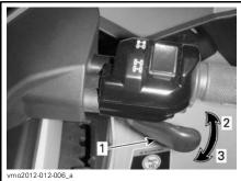
TYPICAL 1. Throttle lever 2. To accelerate
