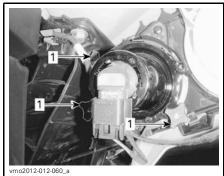
HIGH BEAM ADJUSTMENT 1. Adjustment knobs
