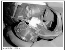
ROTATE BULB COUNTERCLOCKWISE
