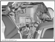
TYPICAL - SOME PARTS REMOVED FOR CLARITY 1. Air filter housing inlet drain tube
