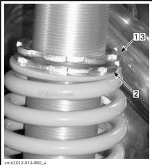
TYPICAL Step 1: Loosen top locking ring Step 2: Turn adjusting ring accordingly Step 3: Tighten top locking ring
