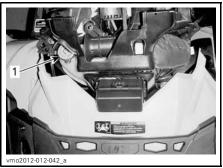
1. Engine coolant reservoir cap
