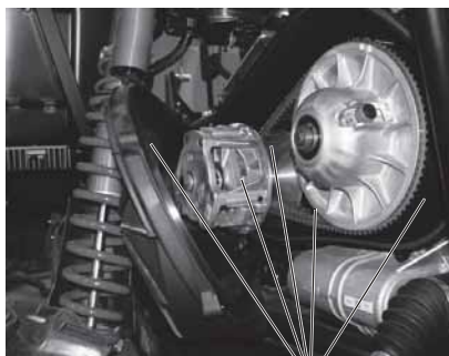
Remove ALL Debris
