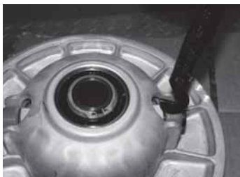
Insert hooked end of tool.
